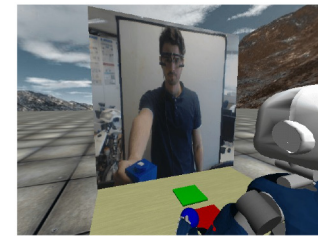
Fig. 13. Experimental setup for the HRI scenario. Human subject is wearing a head-mounted eye-tracker and the relevant objects are present.
